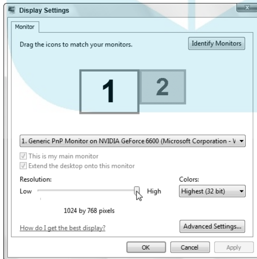
Figure 11-5: Depending on the screen resolution, Windows can squeeze different amounts of information onto your monitor.
